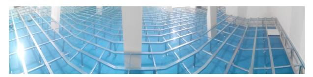
The CONCORDE ISOCON Substructure can be used for all types of Panels. The precision steel Padestals are adjustable in height and protected against corrosion by galvanization. The Padestal base plates are stably glued to the subfloor and can additionally be bolted.
