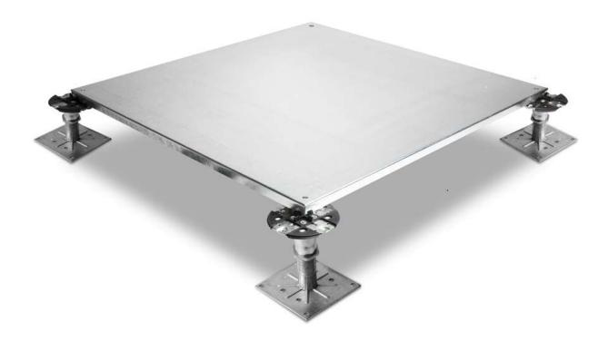
Encapsulated Raised Floor Panel is fully wrapped around by hot dipped galvanized steel. The top and bottom steel sheet is pressed and riveted, high-density chipboard or Calcium Sulphate as inside core. This give high resistant to humidity and have good load bearing properties.
